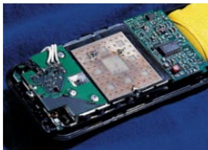
Fractal antennas developed by Fractenna in the US and Fractus in Europe are making their way into cellphones and other devices. Because of their fractal shapes, these antennas can be very compact while receiving radio signals across a range of frequencies.
